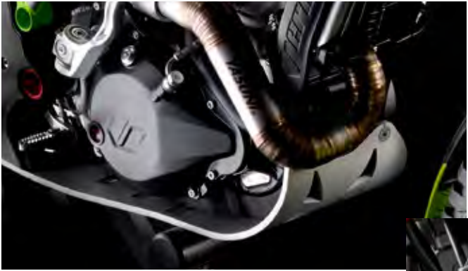
9. NEW CRANKCASE CONFIGURATION FOR INCREASED COMPRESSION.
